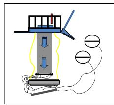
**STEP 2 -** Chute falls to sea with Debarkation Raft and Stabilizer plate attached to bottom, deploying both life rafts with it.
