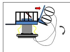
**STEP 1 -** TCAS enters the skid, releases Life Raft retaining strap, cuts lower chute restraint cord with cutting knife which is stowed under the lid of the main chute container, removes large retaining pin from life raft deployment assembly. Extends system deployment lever and deploys system using deployment handle.
