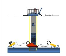
**STEP 3 -** As the debarkation raft descends it starts to inflate, attached to the chute bottom by the anchor cables running through the raft to the stabilizer plate suspended in the water column below the debarkation raft.
